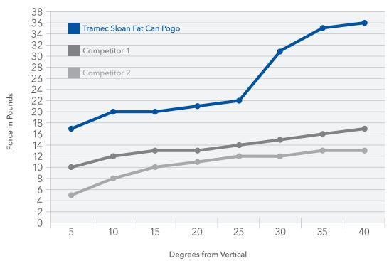
When tested, the Tramec Sloan Fat Can Pogo Stick has outperformed the competition. It has a better ability to handle increasing force when compared against the degrees from vertical. The new spring design provides more resistance along with the necessary flexibility needed to function properly.
