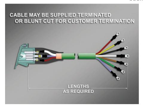
The assemblies are available as standard with the cable end blunt for field termination. Cable ends may also be delivered cut to length with crimped-on ring terminals, solder dipped and encapsulated by melt-lined shrink tube insulators.
