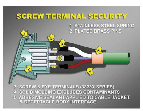
We continue to use materials designed to promote long life with the corrosion proof nylon body. Stainless steel cover springs, and other steel parts with extended life plating. Per SAE recommendations, we continue to provide plated terminal pins. Receptacles are available with a choice of solid or split style pins.
