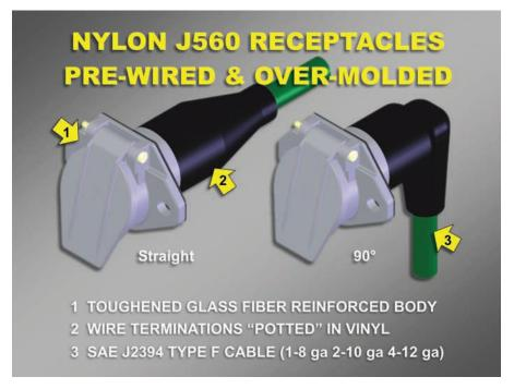
The receptacle is pre-wired with SAE J2394 Type F (flexible stranded) compliant cable. We then place the assembly in a machine and over-
