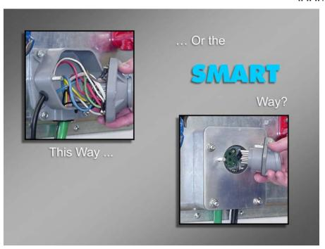
The fleet user gains a receptacle that can be replaced without disturbing the trailer wiring, with minimal labor, and with less chance for error.
