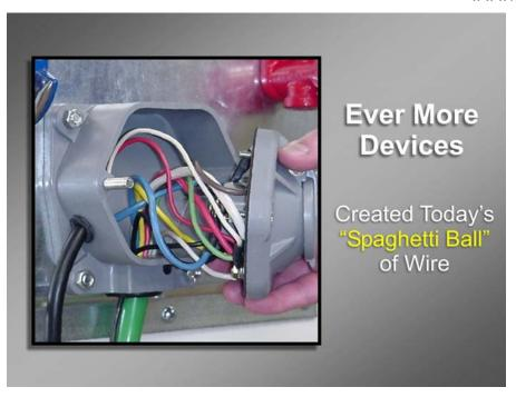
... or by packing the wires into an adapter box. With the advent of ABS, and a few additional lights, the mass of wire to be moved with the receptacle has become a "**Spaghetti Ball**".
