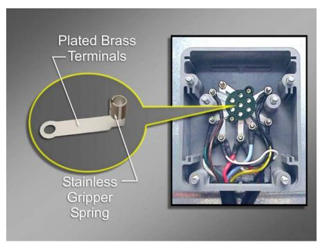
The quality of the electrical connections between the plug-in receptacle and the box is assured by the design of the receiver. Brass buss bars bridge from the harness terminations on the stacking studs to the receptacle pins.
