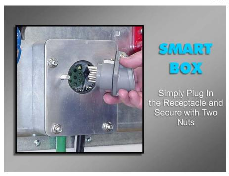
The newly designed J560 receptacle is installed by simply plugging it into the box, and securing it with two nuts.
