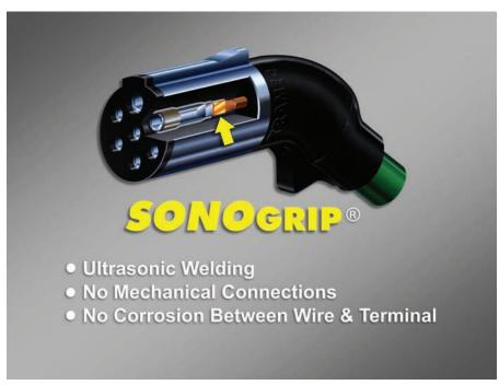
Welding the conductor and terminal eliminates mechanical connections, such as crimping or screw terminals, that can loosen with vibration and thermal shock.
