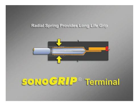
The copper alloy of the terminal stamping provides good electrical properties, while the surrounding band of high-temperature stainless
