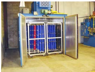
The mandrels that contain the coiled tubing are placed in the ovens to bake so they retain their coil.
