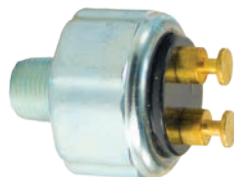
422709 STOP LAMP SWITCH NORMALLY OFF SPST OPERATES 60-120PSI CONTACT CLOSED AT RISING PRESSURE
