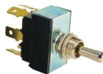
422671 MOM ON/OFF/ MOM ON DPDT 6 BLADES 25 AMPS 12 VOLTS
