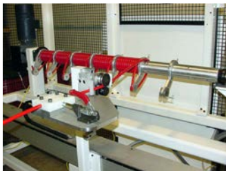
The spooled tubing is wrapped on the mandrel to correct working lengths.
