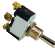
422674 MOM ON/OFF/ MOM ON SPDT 3 SCREWS 50 AMPS 12 Volts
