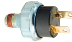
422707 OIL PRESSURE / ELECTRIC CHOKE SWITCH NORMALLY OFF INSULATED SPST ON AT 2-6 PSI
